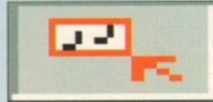
Drag box - make multiple selections, used in combination with the move, copy and erase options
